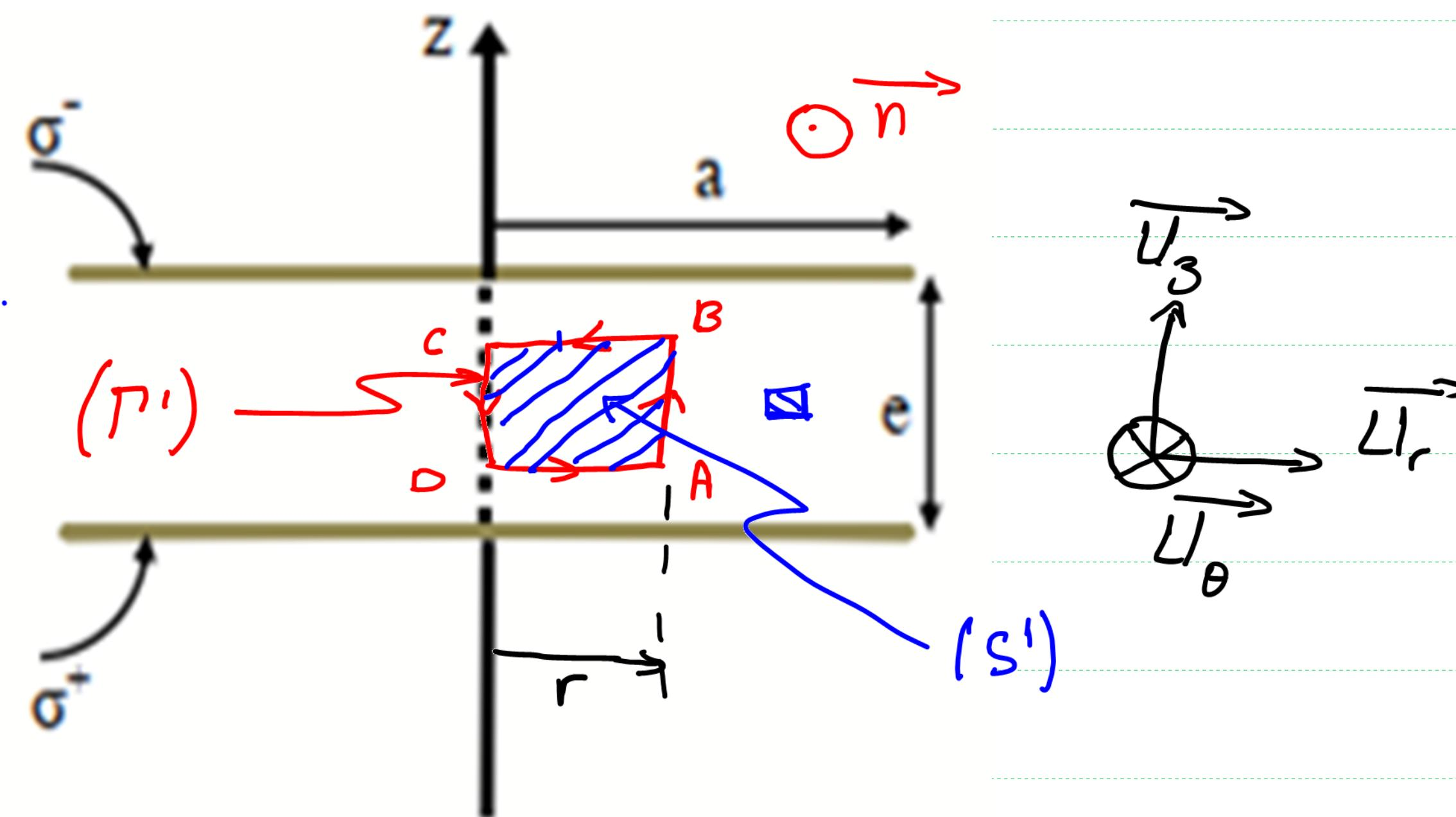
$$\oint_{(\Gamma')} \vec{E}_2 \cdot d\vec{l} = \int_A^B E_2(r, t) \vec{U}_3 \cdot d\vec{l} \vec{U}_3 + \int_B^C E_2(r, t) \vec{U}_3 \cdot d\vec{l}_r \vec{U}_r + \int_C^D E_2(r=a, t) \vec{U}_3 \cdot d\vec{l}_3 \vec{U}_3 + \int_D^A E_2(r, t) \vec{U}_3 \cdot d\vec{l}_r \vec{U}_r$$
